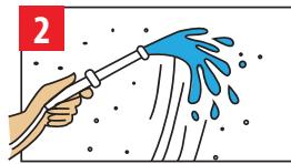
Surface saturation with water (SSD condition)
